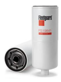
Media Type StrataPore 4.57 inch **Largest OD** 12.32 inch Length 4.736 in Seam OD YES **Standpipe EFFICIENCY, TWA BY SAE J 1985** 98.7% **EMULSIFIED WATER SEPARATION** 95% FREE WATER SEPARATION 95% **MICRON RATING BY SAE J 1985** 7 micron
